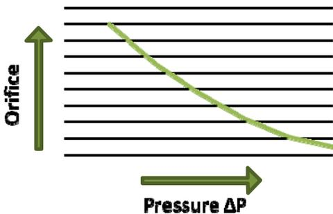
General Relationship of Orifice/Pressure for a Given Flow
